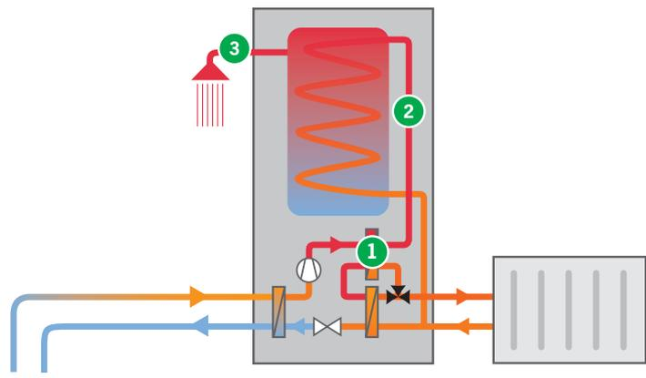
With HGW technology, the temperature in the hot water tank can reach 90 °C. This radically increases the volume of usable tap water.
