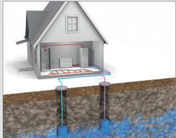
A groundwater heat pump collects energy from the groundwater. The water is pumped up from a water borehole to a heat exchanger, where the energy is recovered.
