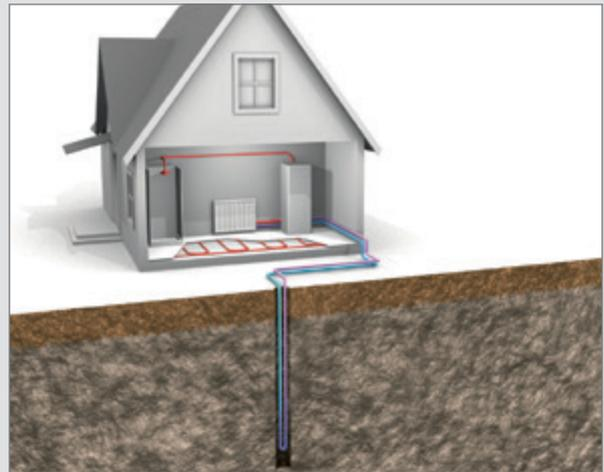
The vertical ground loop collects solar energy stored in the bedrock. A hole is drilled into the bedrock and a pipe is installed to a depth of between 100 and 200 metres. The exact depth depends on the house, size of heat pump and surrounding conditions.
