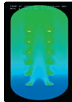
TWS hot water tanks are specially designed for heat pumps. The technology layers the hot water in the hot water tank so that the heat can be used in the best way. (In the photograph, the hot water is represented by the green colouring and cool water by the blue.) The amount of energy used to create hot water by TWS could only create lukewarm water in a conventional hot water tank.
